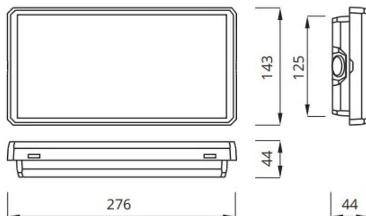
**WYMIARY OTWORU MONTAŻOWEGO (mm):**
