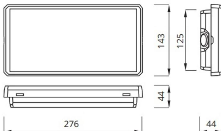
**WYMIARY OTWORU MONTAŻOWEGO (mm):**
